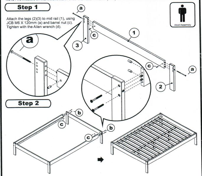
Attach bed frame assemblies to the head rail assemblies, using JCB M6 X 70mm (b) and barrel nut (c) as shown. Tighten with allen wrench (d). For Slat kit assembly, follow assembly instructions included with slat kit.
