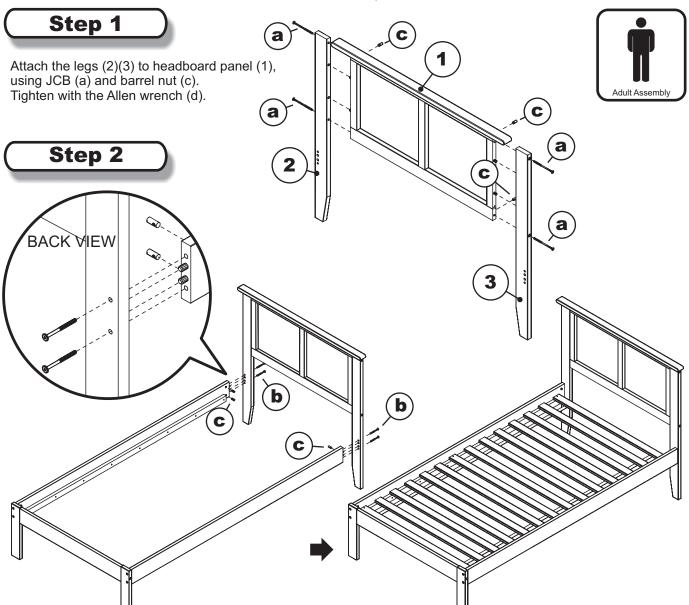
Attach bed frame assemblies to the headboard assemblies, using JCB M6 X 70mm (b) and barrel nut (c) as shown. Tighten with allen wrench (d). For Slat kit assembly, follow assembly instructions included with slat kit.
