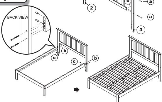
Attach bed frame assemblies to the headboard assemblies, using JCB M6 X 70mm (b) and barrel nut (c) as shown. Tighten with allen wrench (d). For Slat kit assembly, follow assembly instructions included with slat kit.
