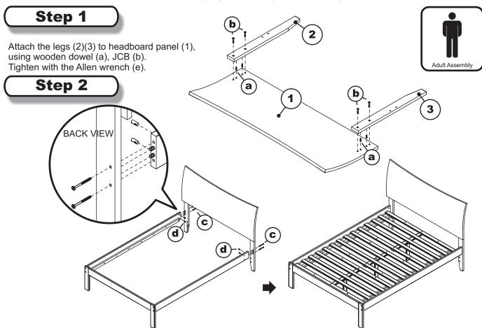
Attach bed frame assemblies to the headboard assemblies, using JCB M6 X 70mm (c) and barrel nut (d) as shown. Tighten with allen wrench (e). For Slat kit assembly, follow assembly instructions included with slat kit.
